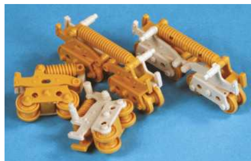
A combination of TMD and Tamiya parts to produce the suspension units.
