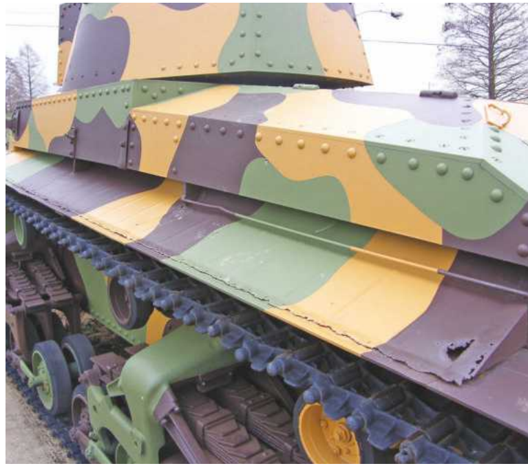
Air intake for the engine is via louvres along the sides.
