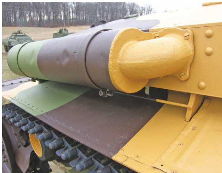
ABOVE: Close-up view of the vehicle's single exhaust silencer. BELOW: A close-up view of the rear engine access doors.
