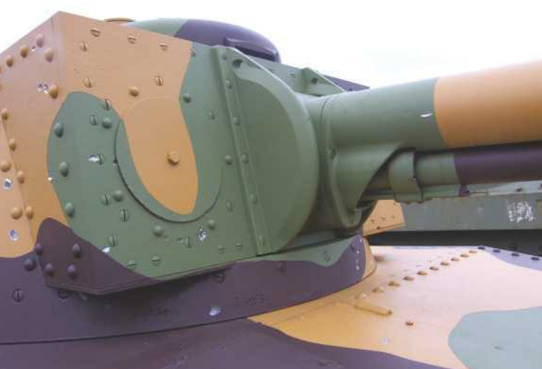
ABOVE: Close-up of the turret front; note the various silver-highlighted bullet scars.
