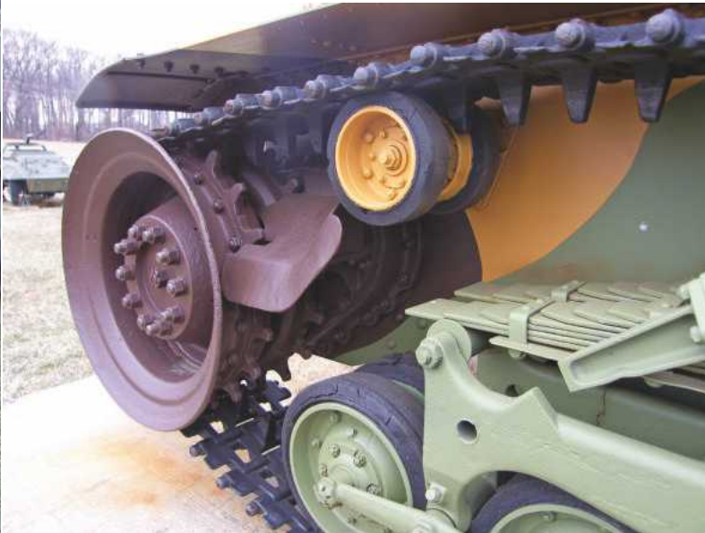
My guess is that the blade mounted forward of the sprocket was meant to keep mud from building up inside the running gear.
