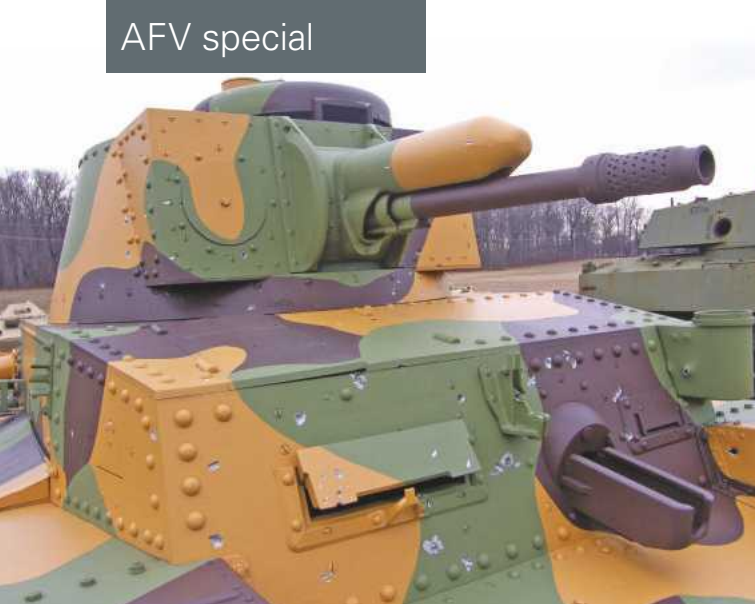
ABOVE LEFT: The 37mm A3 gun was mounted with a very distinctive recuperator cylinder above the barrel. Combined with the geared elevation and traverse the heavy mount should have meant that it was a stable gun platform.
