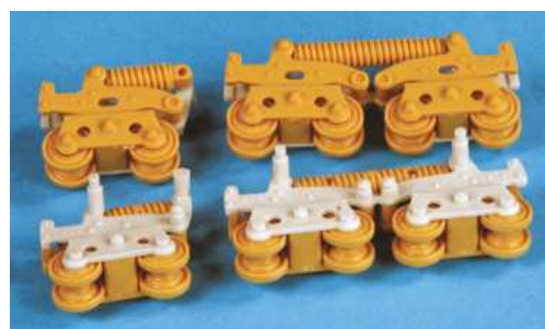
A combination of TMD and Tamiya parts to produce the suspension units.
