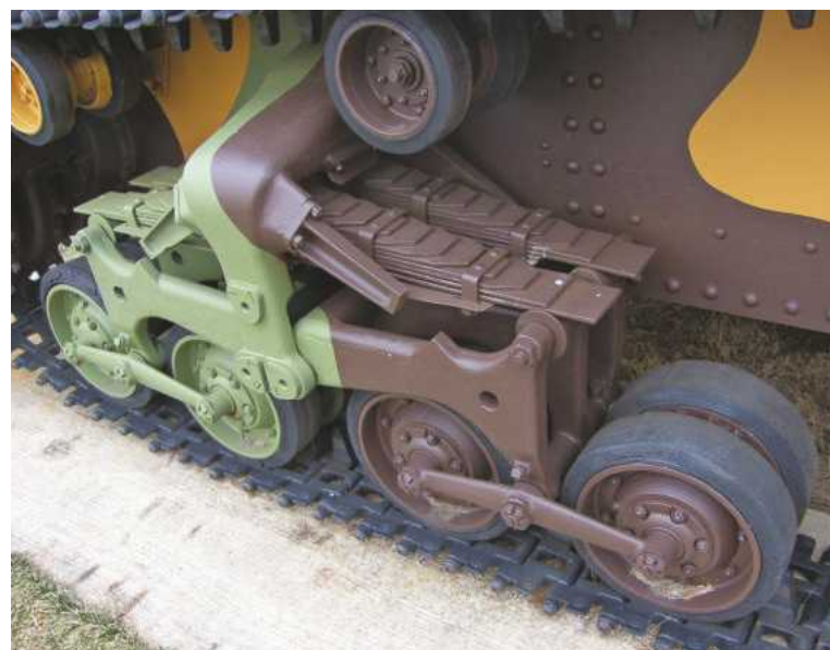
The suspension was effective, apparently giving a smooth ride and extremely good hill-climbing ability.
