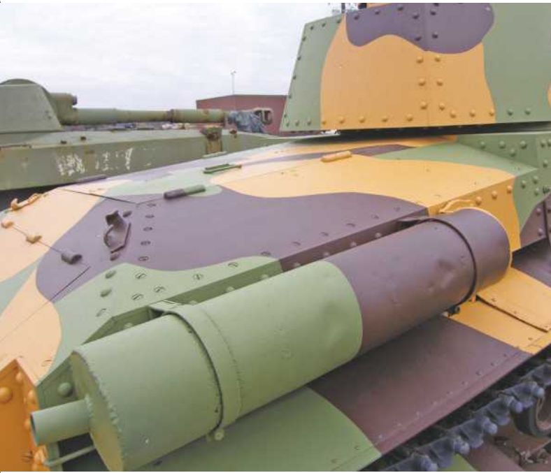
A single exhaust silencer is fitted to the right-hand side of the engine.
