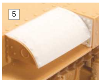
PHOTO 5: The scratchbuilt radiator air intake cowl in place. Note where the section of the original right rear sponson plate has been used to form the rear of the cowl (as it should).
