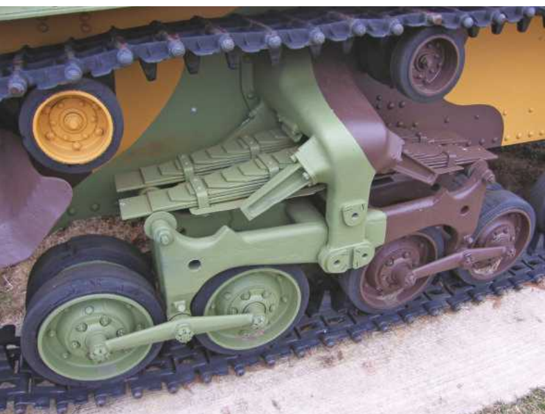
I believe that the suspension design may in part at least derive from a Vickers design used on their 6-ton tank.
