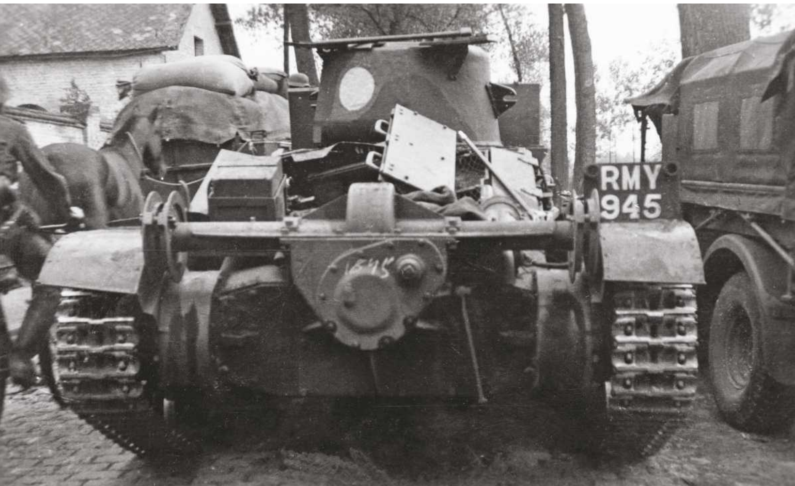
ABOVE: From the front Gourock appears to be a typical A11 waiting to be towed away. The rear view shows the fitting for the Fowler Coulter Plough though the plough itself is not in place, this can just be seen in the other photo. Note the Unit Serial Number 1875 painted on the plough fitting.
