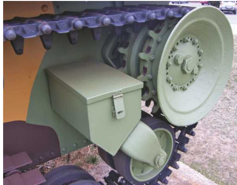
My guess is that the blade mounted forward of the sprocket was meant to keep mud from building up inside the running gear.
