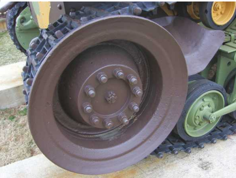
The rear drive sprocket has this unusual dish around it.
