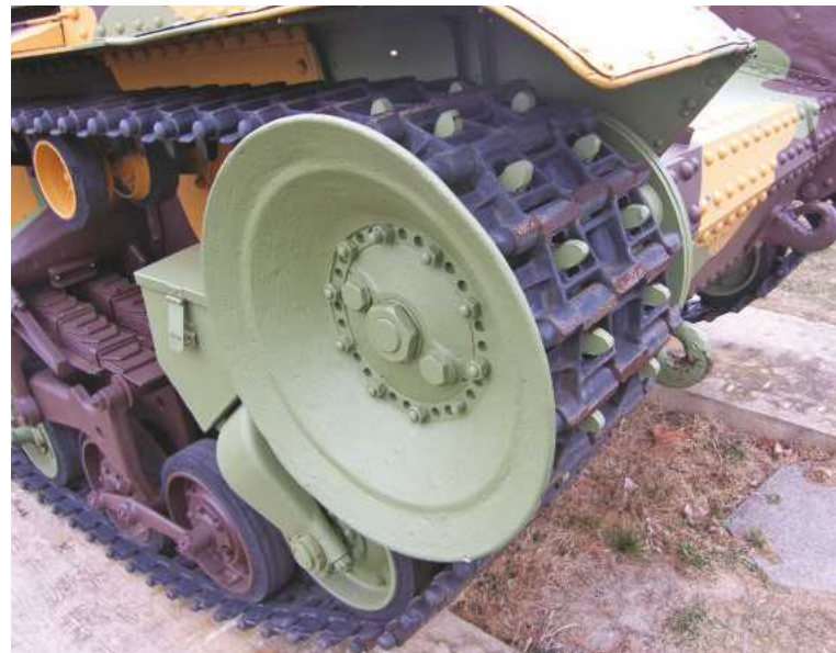
The LT Vz 35 featured unusual toothed front idler wheels; these were not driven.
