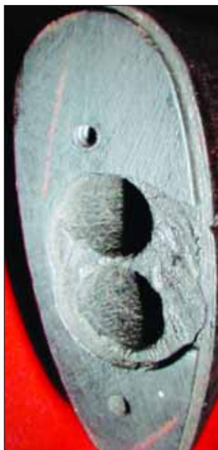
Similar routing hacked at to make room for the butt plate hinge at the edge.
