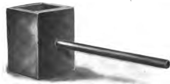
Fig. 8. Form of Hollow Cast Iron Block used for Test.
