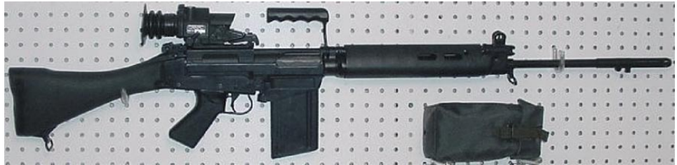
Figure 6. The British 7.62 mm L1A1 Self-Loading Rifle. Accurate and powerful, but its ammunition weighed twice that of 5.56 mm. the SLR suffered from considerable recoil and could not be controlled when fired in automatic mode from the shoulder, a disadvantage that led to a deletion of its automatic fire capability. (Source: Max Popenker)
