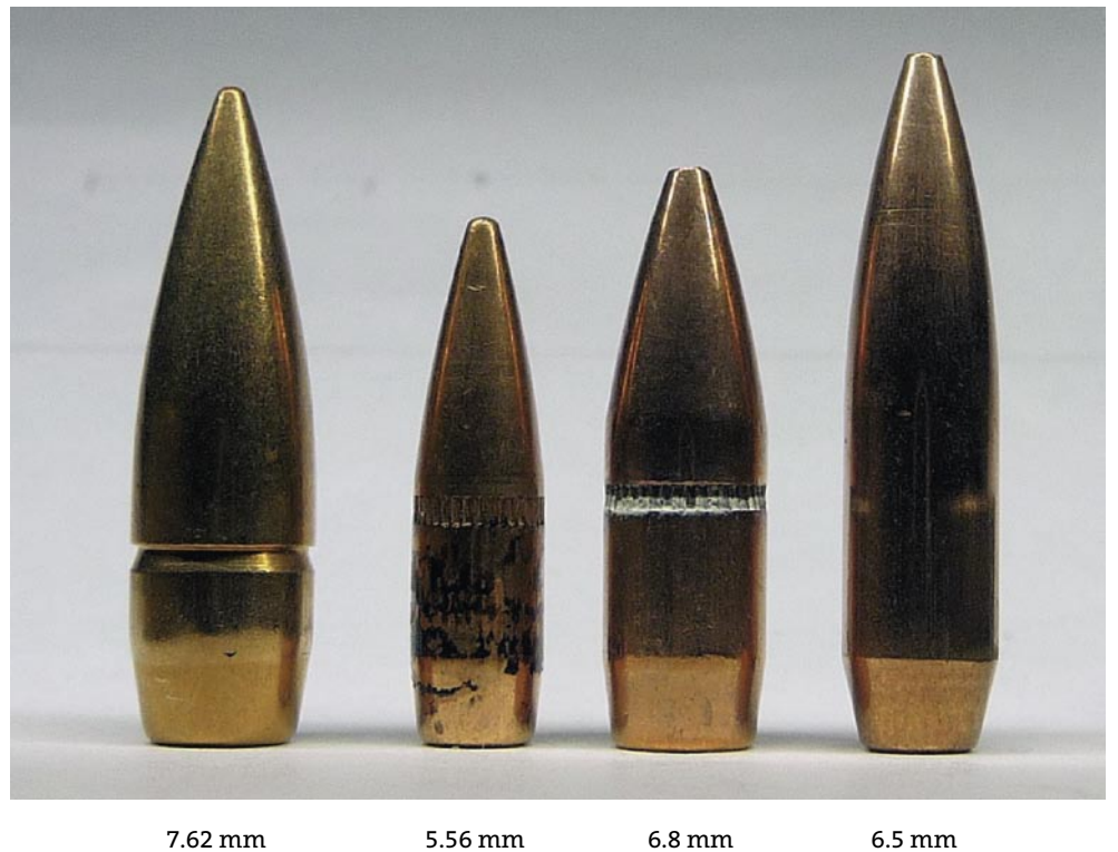
Figure 11b. Comparison of bullets discussed with weights and lengths, (from left to right): 7.62 mm NATO (9.5g, 28 mm), 5.56 mm NATO (4.1g, 23 mm), 6.8 mm Remington SPC (7.5g, 25 mm), 6.5 mm Grendel (7.8g, 30 mm). (These weights are from measured examples and may differ slightly from others quoted in this report.) The length of the 6.5 mm bullet accounts for its excellent aerodynamics and long-range performance.
