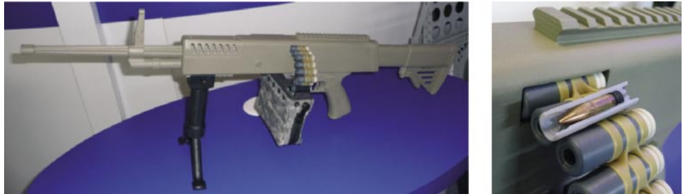
Figure 12. LSAT prototype machine gun with plastic-cased and (sectioned) caseless ammunition (Source: Anthony G. Williams)
