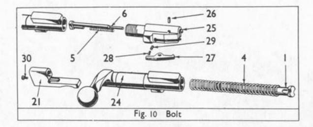
36. To Strip Bolt (Fig.10). - Unscrew the bolt head (25), and pull out the firing pin (6) and firing pin spring (5). With a suitable punch, drive out the extractor pin (26); remove extractor (27), extractor plunger (28), and extractor spring (29). Remove the striker screw (30) from the cocking piece (21), and unscrew the striker (1) with the "Tools Striker No.2" as used with the No.4 rifle. Remove striker and striker spring (4) from the bolt (24).
