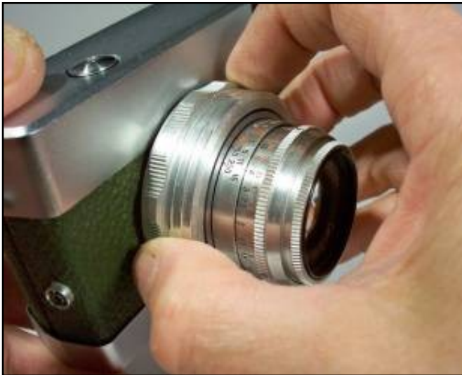
Image 3: Film winding and shutter cocking ring. © 2012 Gordon Risk
