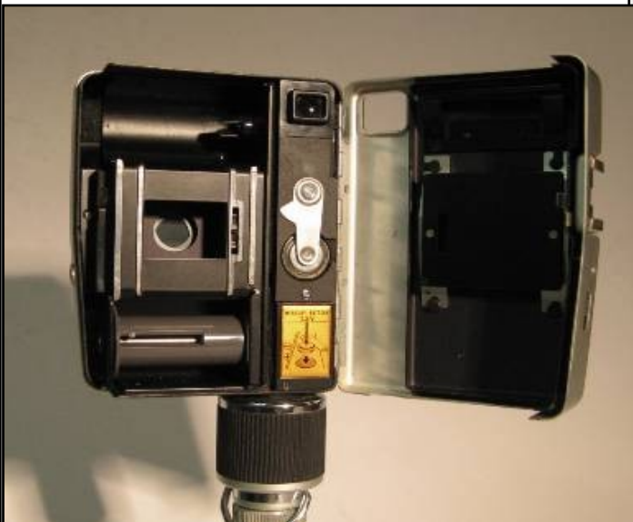
Figure 5: Vertical Film Transport, Canon Dial © Gordon Risk
