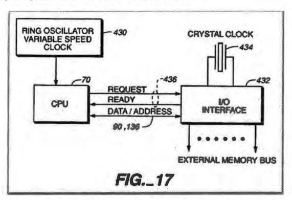
Id. at Fig. 17. In the illustrated embodiment, CPU 70 operates asynchronously with I/O interface 432. ID at 7 (citing Technology Stipulation at 2.) I/O interface 432 is controlled independently by crystal clock 434. Id. The on-chip ring oscillator variable speed clock 430 clocks the CPU 70.
