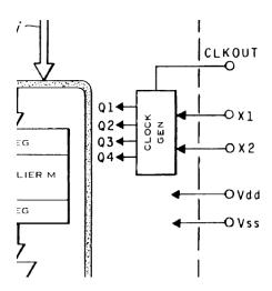
A5462 (Magar, Fig. 2a). Magar's "clock gen" block in Fig. 2a includes circuitry to divide the oscillating signal generated by the external crystal to provide a timing signal to the CPU:
