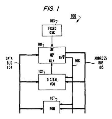
A5495 (Sheets, Fig. 1). As with Magar, the applicants distinguished Sheets based on the location of the component that generates the clock signal that clocks the CPU. The claimed invention requires an on-chip oscillator to generate the clock
