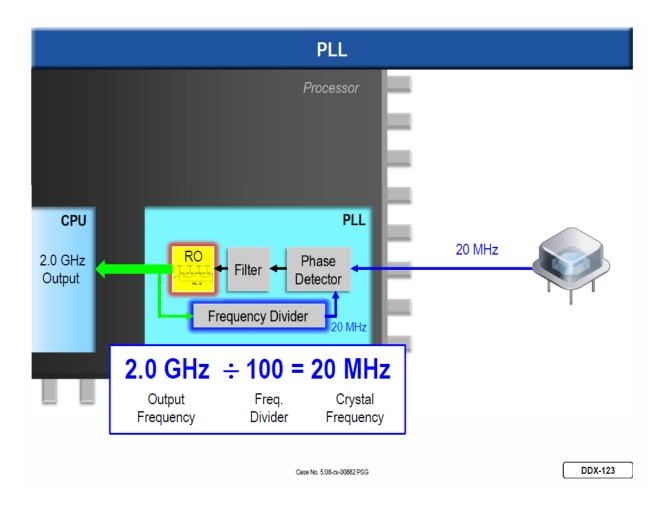
A7859-60; *see also* A8666 ("Q. So you've got a 2.0 gigahertz clock signal generated by the ring oscillator that's clocking the CPU, and you divide by 100, and that's what this circuitry actually does; correct? A. Yes.").
