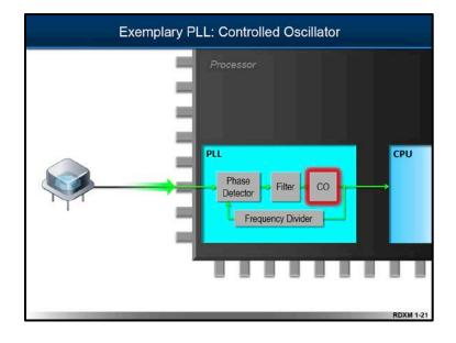
The **CO**" in the diagram) is a ring oscillator that generates a very high frequency clock signal (*e.g.*, 2.0 GHz), which is used to clock the CPU. A sample of the high frequency clock signal from the **CPU** is also divided by the **Frequency Divider** to obtain a much lower frequency
