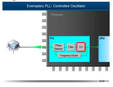
RDXM 1-21. Because the CO/ drives the CPU, any change in the rate of the CO/ 's oscillation will cause a corresponding change in the processing frequency of the CPU. In other words, the processing frequency of the CPU <u>is</u> the rate (or speed or frequency) of the clock signal from the "entire oscillator" (**DD**) that drives the CPU.
