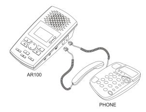
To connect in handset mode, simply remove the curly cord from your telephone base and connect into the Call Assistant SD and connect the short handset lead supplied between the telephone handset socket and the Call Assistant SD as shown above.
