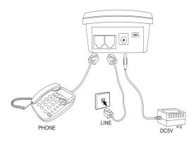
Disconnect the telephone line cord from the base of your telephone (the other end connects to wall socket) and plug this into the Call Assistant SD. Connect the long cord supplied between the Call Assistant SD and the socket on you phone (where you removed the line cord). NOTE: The Call Assistant SD will record calls when connected to the phone line, it is
