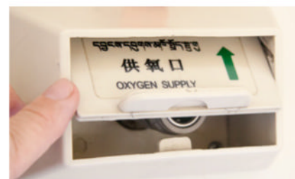
Oxygen outlets are provided beside seats in the passenger cars, which are unpressurized.
