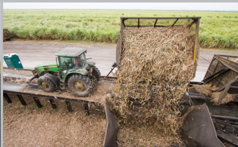
2 Tractor-hauled trailers dump cane onto a large conveyor to load railcars in November 2014.
