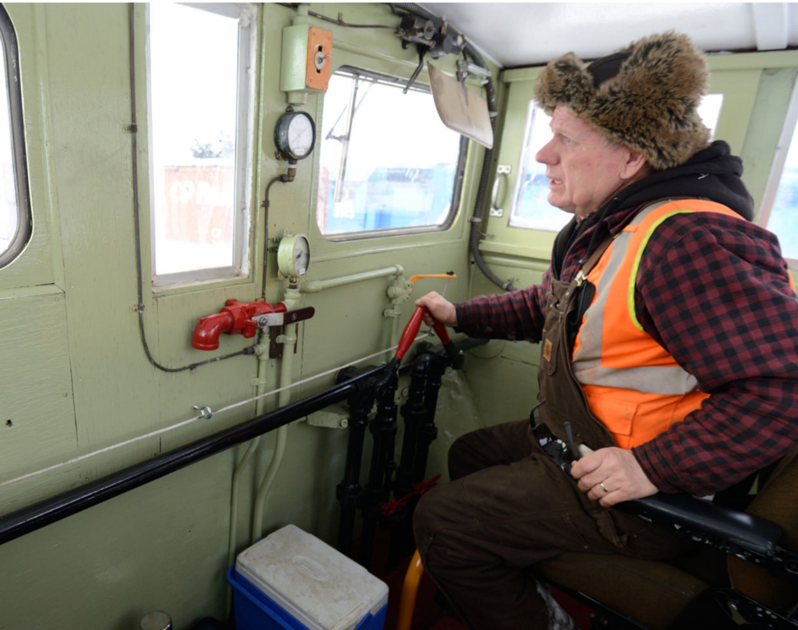
Looking to the rear of the plow on the Ontario Southland near St. Thomas, Ont., one moment you see FP9 No. 6508, and the next you don't. Below, foreman Jack Hyde retracts the wings inside plow No. 401005. His vantage point is the cupola on top of the plow.
