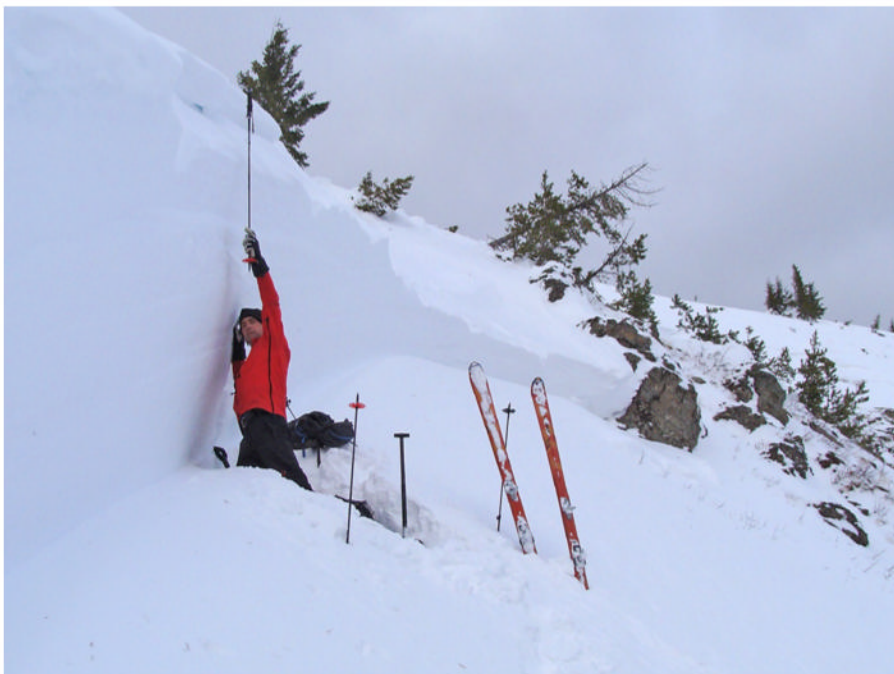
To create avalanche forecasts, Ted Steiner and his associates hike, ski, or snowshoe onto the slopes above BNSF's line over Marias Pass to examine the area's snowfall. At right, Mark Dundas uses a shovel to perform a compression test, finding out how much pressure the layers of snow can withstand before collapsing, which helps determine how likely the snow is to slide. Two photos, BNSF Railway
