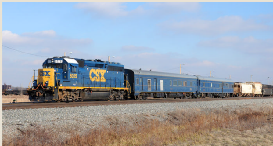
A two-car CSX Transportation track inspection, or "geometry," train scours the former Baltimore & Ohio main line at Defiance, Ohio, in January 2011. Brian Schmidt
