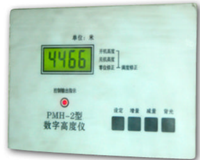
This altimeter did not display the correct altitude for Tanggula Pass, 5,072 meters or 16,640 feet. Two photos, Albert Tay
