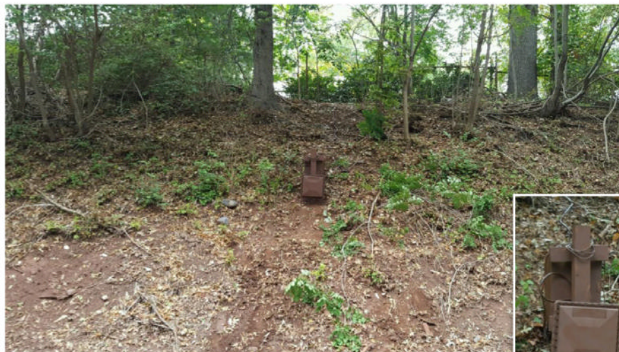
Railroaders found this brown-painted automatic equipment identification, or AEI, reader along a railroad right-of-way in New Jersey. Three photos, Association of American Railroads
