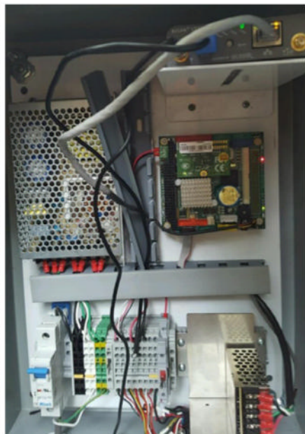
The computer and other components of an equipment box supporting an AEI freight car tracker in New Jersey.
