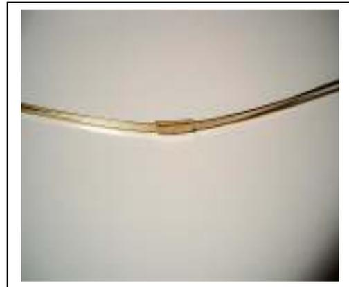
Now the fun stuff, bending the wire (bail). Here we'll use the needle-nosed pliers to get the proper bends. Once again, some people wrap the nose with masking tape. Did I mention that I'm hard core? Oh, the pliers ..... Notice that I place the tip of the pliers tight against the binding wrap
