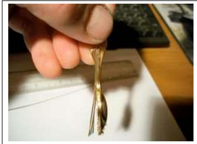
**Time for the next binding, this is where everything will start to come together. I start mine between the wires as shown because I don't crimp this binding and this will keep the binding from unwrapping. Again, these should be tight and uniform...**
