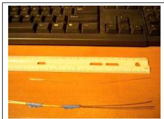
**Now we're ready to start wrapping. It's important to go slow, keeping the wraps tight and uniform. Uneven bindings will make your work of art look like the work of a madman with wire. The ends of the binding wire can be tweaked after you get the on...**
