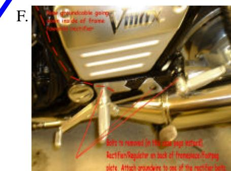
F. Bolts (on picture peg) to remove frame plate. R/R mounted on the inside. Attach the ground wire to one of the bolts holding the rectifier. Clean the R/R and contact area. Fine tune the cable layout and use plastic wraps to secure cable.
