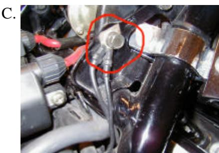
D. Mount new improved cable to engine ground and frame ground, use plastic wraps to secure cable to frame.
