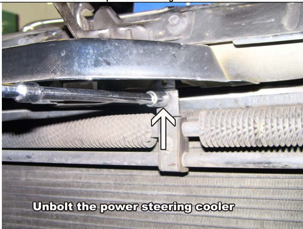
Unbolt the power steering cooler from bracket
