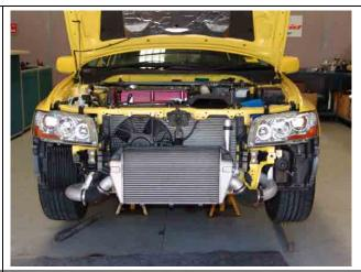
remove standard front mount intercooler and intercooler pipes
