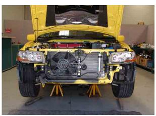
install front hdi bracket and intercooler lower bracket.
