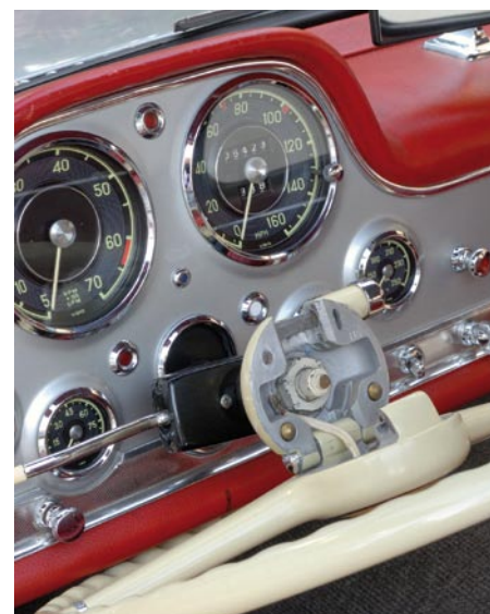
△ The steering wheel moves to help the driver get in/out.
