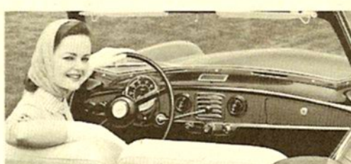
METROPOLITAN instruments are clustered directly in front of the driver for easiest reading. Gear shift lever is mounted on the steering post.
