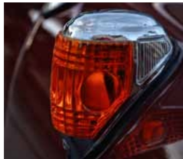
ABOVE Direction indicators are mounted on the top of the Ponton’s front wings.
