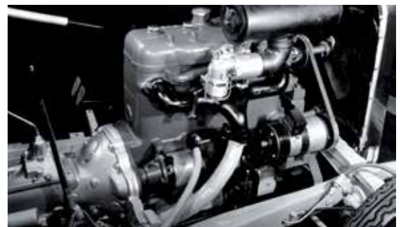
ABOVE Engine was a 2.5-litre four-cylinder delivering 44bhp and 26mpg.
