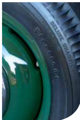
BELOW Skinny 16-inch wheels have vintage compound Firestone cross ply tyres.
