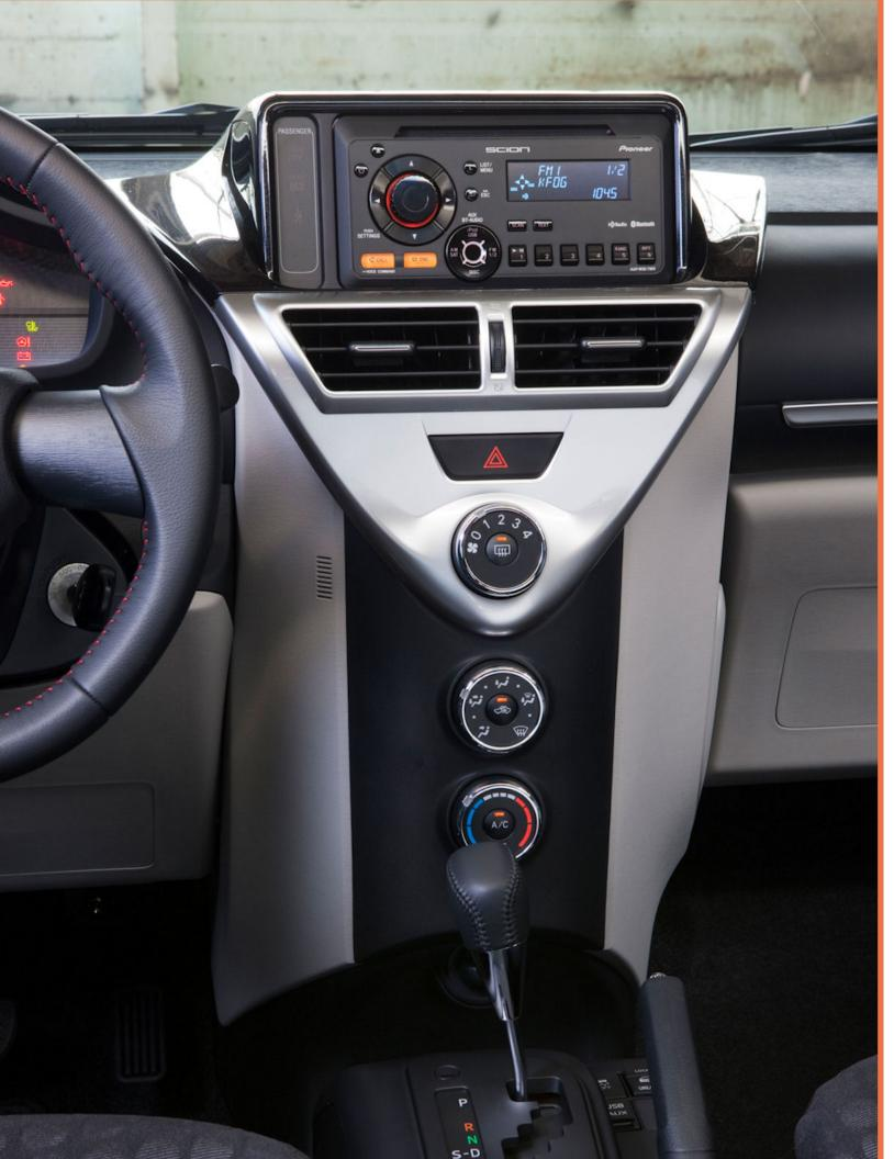
The other major difference between the two vehicles is that the iQ is equipped with a CVT transmission, and the ForTwo is equipped with a herky-jerky automated manual transmission.
