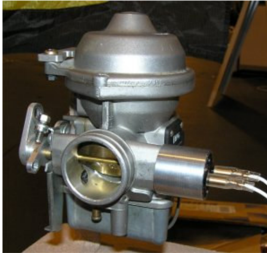
Ice Eliminator installed
