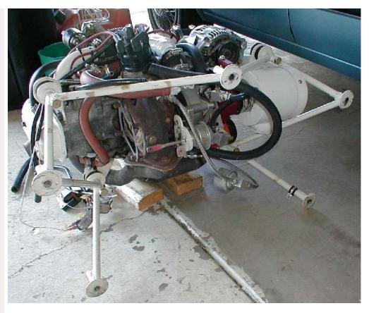
Cruise between 3300-3500rpm and burned approximately 4-5gph. Without using any boost the aircraft performed similarly to the 70HP Revmaster that was previously installed so I approximate the output at 65-75hp. With boost the aircraft performed better than previously so I approximate the output at 80-90hp. Total weight of all included components is approximately 206 pounds.
