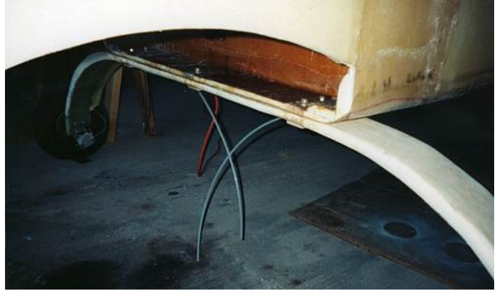
Photo of hoop gear leg attachment using bolts
