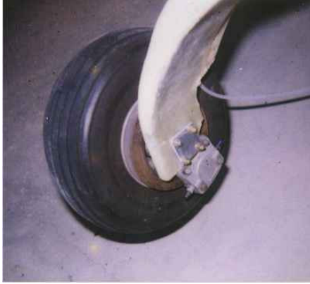
My installation of Cleveland brakes and wheels on the hoop gear.
