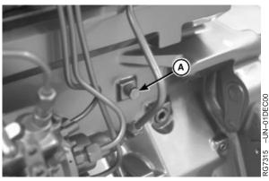
Engine Block Drain Valve
