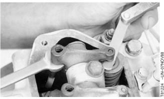
Checking Valve Clearance
