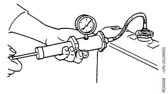
Pressure Testing Cooling System
