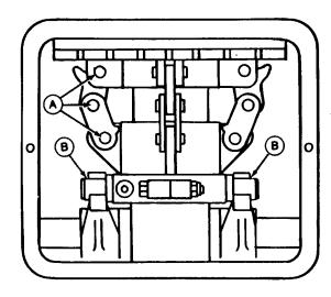
Lubrication Internal Parts of PTO Clutch
