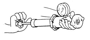
Pressure Testing Radiator Cap
