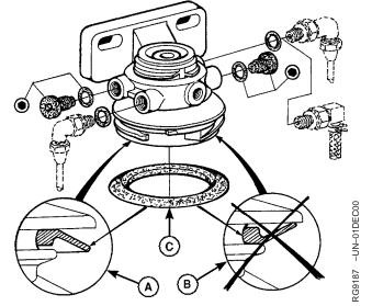
Fuel Filter Dust Seal Installation
