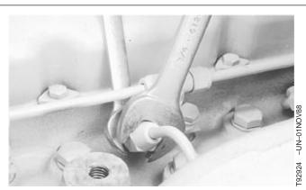
Bleeding Fuel System at Injection Nozzle
