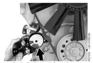
Checking Belt Tension with Tension Gauge
