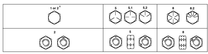
Top, SAE Grade and Head Markings; Bottom, SAE Grade and Nut Markings
