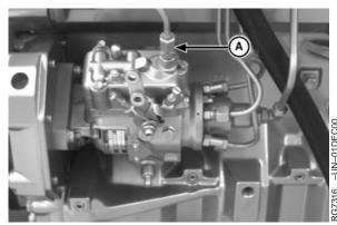
Fuel Supply Line Connector at Injection Pump
