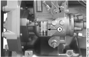
Injection Pump Serial Number Plate
