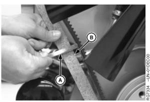
Checking Belt Tension with Straightedge
