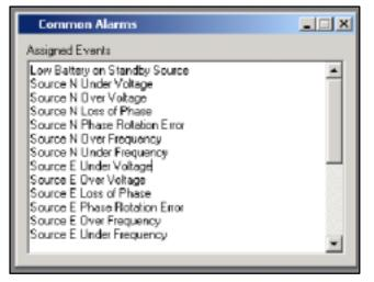
Figure 3-30 Common Alarms Display
