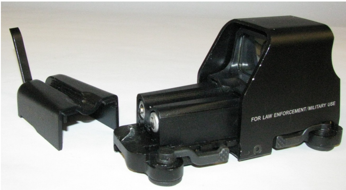
Figure 9(a): Battery compartment of a genuine Model 553 L-3 EOtech holographic weapon sight.
