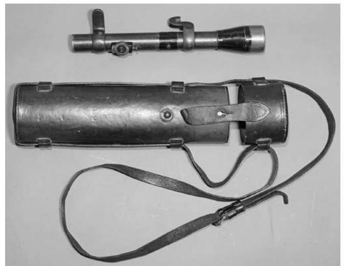
Figure 1. The Watts telescope. This particular example bears Purdey mounts more usually associated with the Aldis 'scope.
