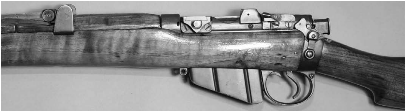
Figure 2. Side view of Short Magazine Lee Enfield rifle fitted with bases for the William Evans telescope.
