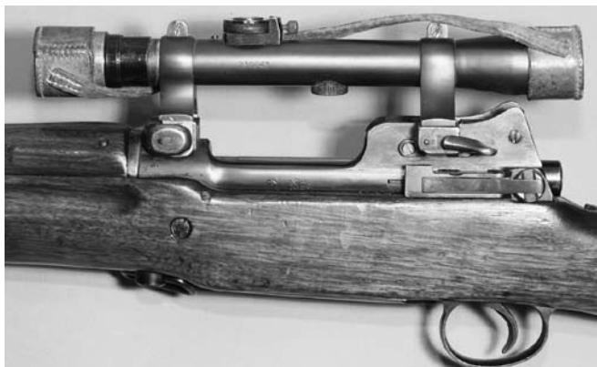
Figure 6. Side view of the receiver area of a Pattern 1914 sniper's rifle equipped with the Model 1918 telescope
