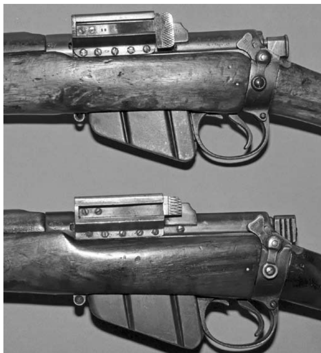
Figure 4. Two Periscopic Prism Company rifles with scopes removed in order to show the two minor but distinct variants of mount base encountered.
