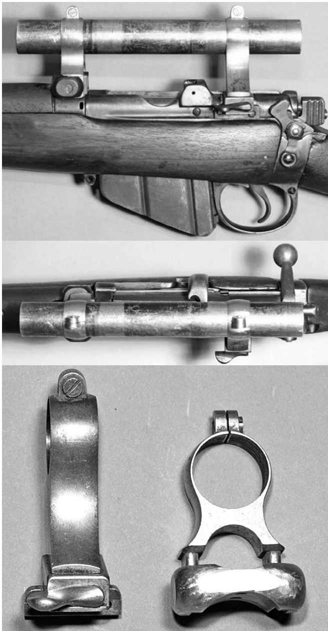
Figure 6. Over bore claw mount system as used with later Aldis telescopes. A similarly-sized length of mild steel rod is shown in place of a missing telescope..
