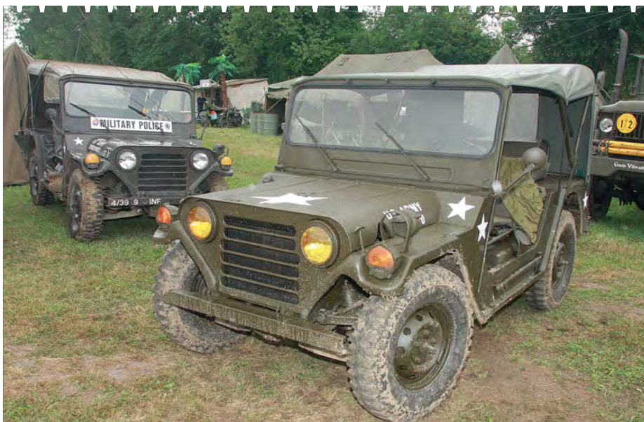
The M151A2, introduced in 1970, was a revised version of the M151A1 that incorporated redesigned suspension to reduce rollover accidents
