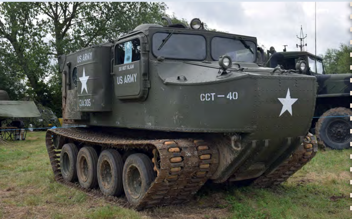
ABOVE: It is thought that there are fewer than ten fully operational M76 Otters in the world ABOVE LEFT: The tracks were an evolution of the type found on the Weasel, a single long rubber band with added metal cleats and thicker rubber blocks BELOW: A 70 gallon fuel capacity gave a approximate 200 mile road range
