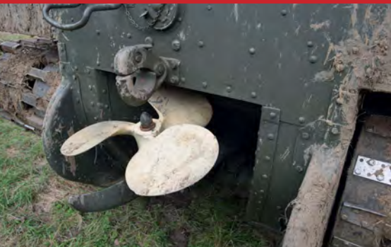
When not in water, the propeller folds up neatly to avoid snagging on the ground
