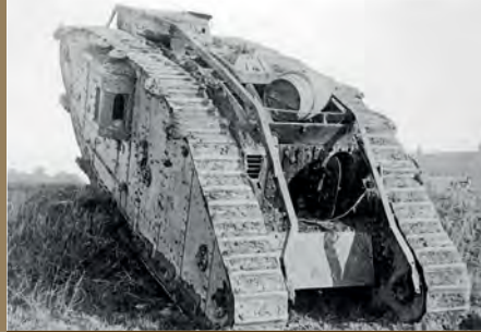
Abandoned at Cambrai is this unidentified Mk IV. The large rail running over the top would carry the unditching beam. The second rail appears to be partially missing
