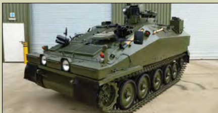
Spartan CVRT Dieselised APC , Fitted Cummins BTA 5.9lt Turbo diesel engine, Engine: power 195 hp, David Brown TN15d Epicyclic Semi-Automatic Gearbox with Neutral turn capability, Max road speed 72 km/h, Range 750 km, Manoeuvrability, Gradient 60%, Side slope 35%, Vertical step 0.5 m, Trench 2m, Fording 1m etc, Ex condition, ..... Guide price from £19,995 (1 Available)
