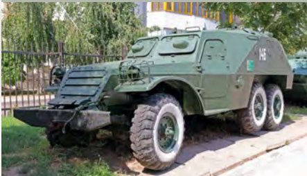
A BTR-152K six-wheeled Soviet Armoured Personnel Carrier built on the chassis and drive train of a ZIS-151 utility truck
