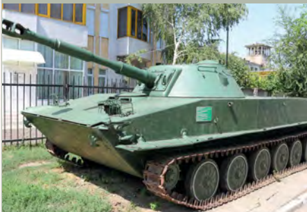
A Soviet amphibious light tank PT-76 that was introduced in the early 1950s and soon became the standard reconnaissance tank of the Soviet army
