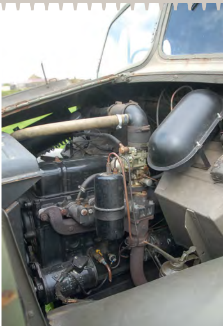
ABOVE: The Bedford OXD's six-cylinder WD OHV 3,519cc petrol engine is simple to maintain though ignition coils failing are a problem at the moment
