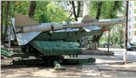
The Soviet S-75 Dvina (SA-2 Guideline) is a surface-to-air missile defence system.
