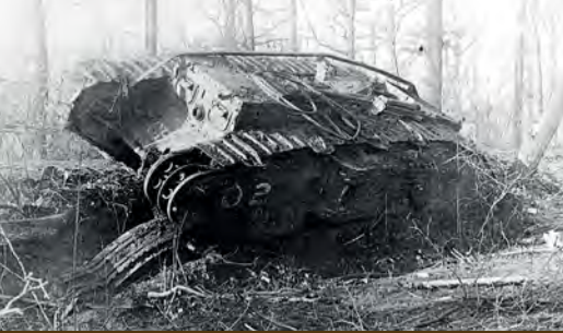
The tank 'Ceylon' became stuck at Bourlon wood on November 23. While trying to free itself it broke a track and was abandoned by its crew
