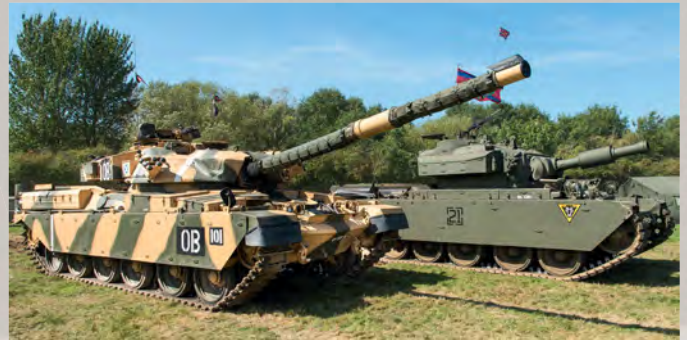
Chieftain (left) entered service in 1966 was a development of the Centurion. It's rifled Royal Ordnance L11A5 120mm gun became the new NATO standard calibre. Centurion (right) introduced in 1945 and was the UK's primary MBT of the post World War Two period.
