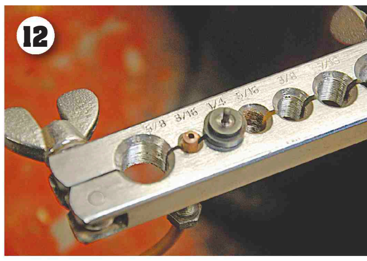
12 While not forgetting to fit the threaded coupling first, the pipe can then be gripped in the flaring clamp. The amount the pipe stands proud of the clamp should be the same as the depth of the head of the forming tool (shown on the right).
