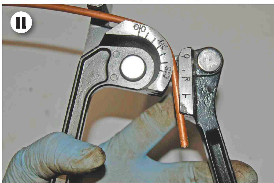
11 For neater curves the bending tool is simple to use, can handle several different diameters of pipe and is marked in degrees so the pipe is bent accurately.
