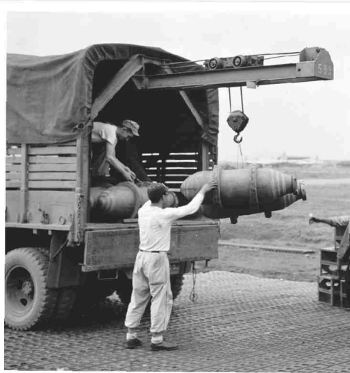
The bomb service truck was furnished with a canvas cover for the cargo bed and the design of the truck was such that the cover did not interfere with the bomb handling operation.
