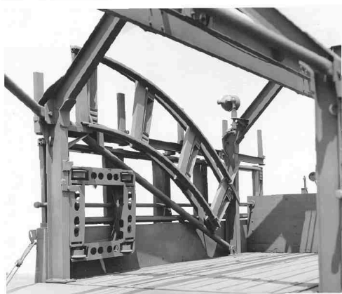
Stowage for the curved track section as well as a dolly was provided on the inside bed sidewall of the M27B1.
