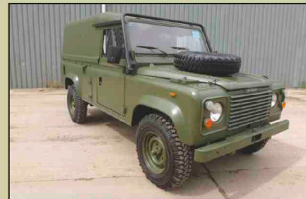
Land Rover Tithonus 110 Defender Hard Top , Fitted 2.5ltr NAD engine, 5 speed gear forward and one reverse gear box, Hi/Low transfer box, Centre Diff lock, Front disc brakes, Rear drum brakes, etc., mileage from 22,000 kms, Excellent condition, Guide Price for RHD £5,000 to £8750, Guide Price for LHD £6,500 to £8,500 (20 Available)
