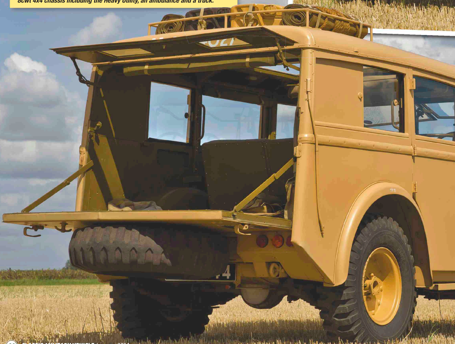
Below: During WW2, Humber produced a range of vehicles based on the same 8cwt 4x4 chassis including the Heavy Utility, an ambulance and a truck.
