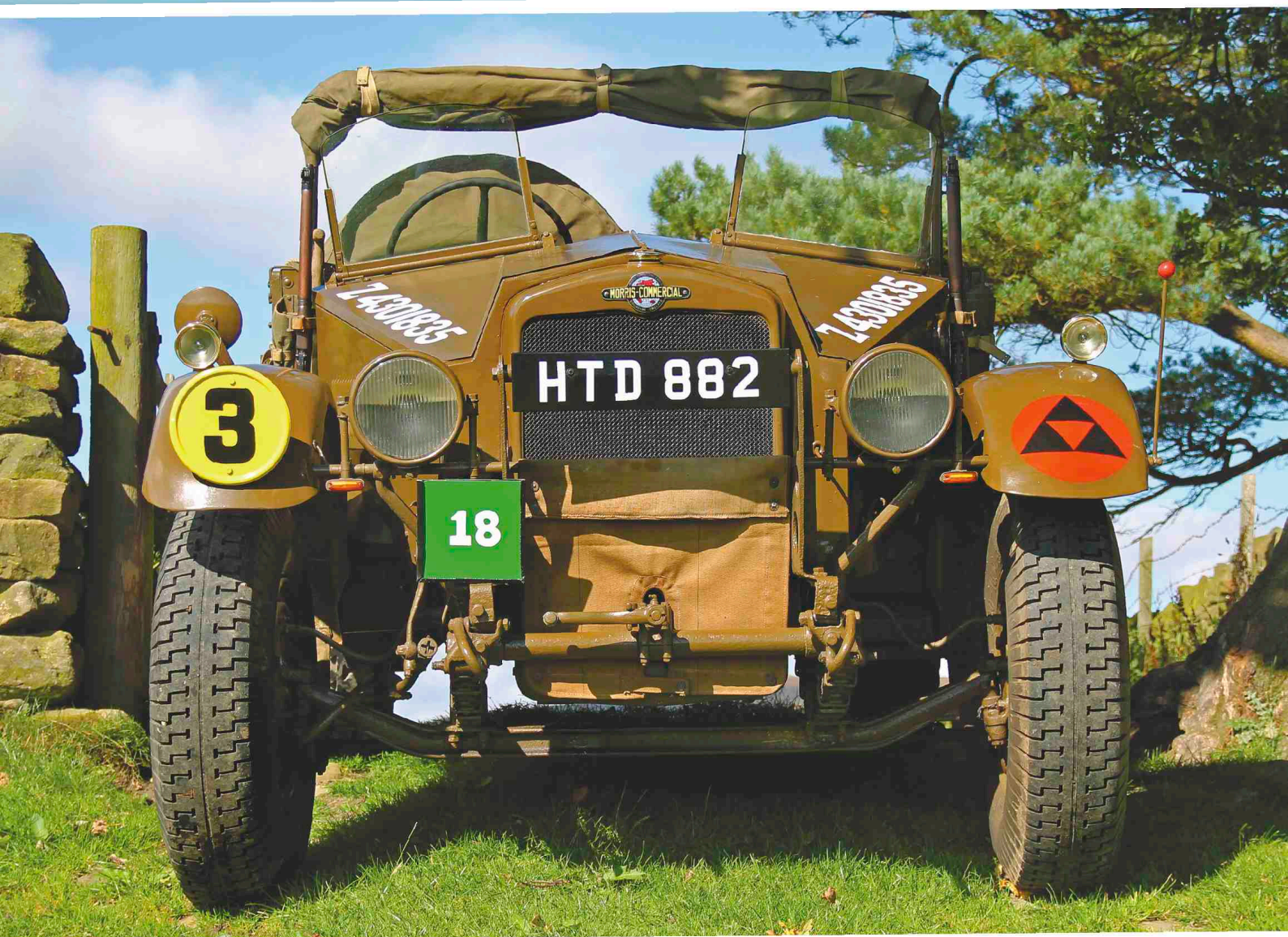
Above: The markings are for a vehicle serving with the 2nd Battalion of the East Yorkshire Regiment. The red circle with black triangles indicates attachment to the 3rd Division. Right: It is believed that the CS8 left the factory as a two-pounder anti-tank gun portee but was converted into a general service truck, perhaps before even being issued to a unit.
