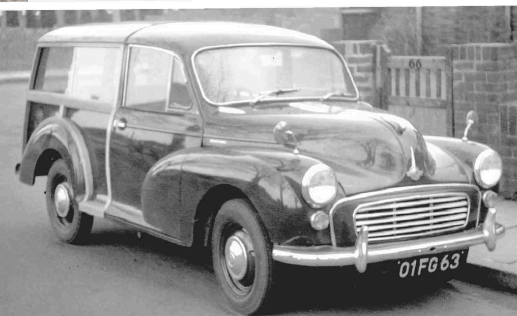
Army Traveller 01FG63 fitted with overrides, which were not normally fitted to military Travellers. Note the round chrome wing mirrors.
