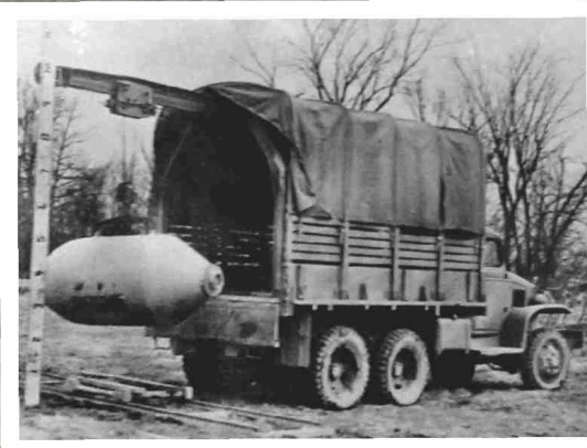
Above: On the first prototype, the hoist rode on the lower flange of an I-beam. The truck is shown here placing a bomb on the dolly and track supplied with the truck. Left: A trio of US Air Force CCKW bomb service trucks pick up their deadly loads of 2000 lb (909kg) bombs at a dump in Japan on 17 June 1953. These bombs are destined for Korea.
