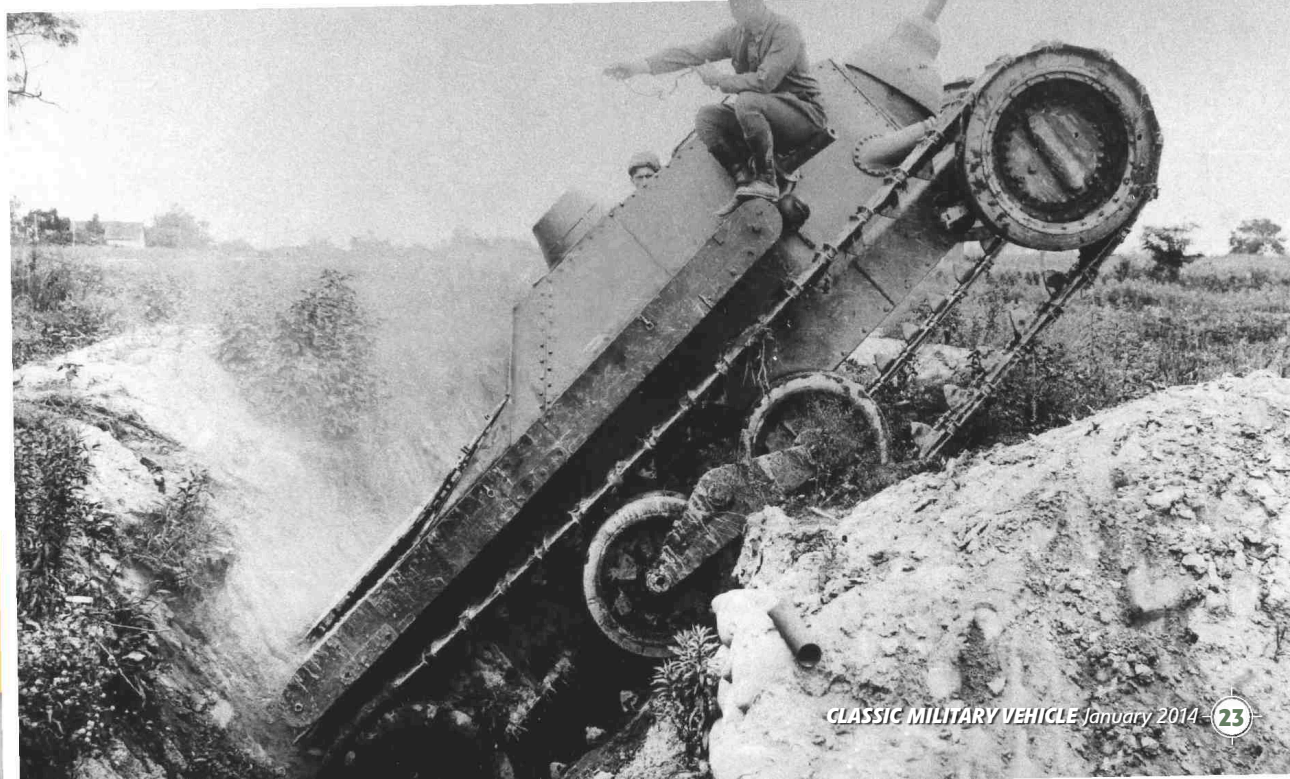
From the rear M1922 looks particularly unusual and the length of the rear track frames becomes obvious. This would be a typical Johnson feature, whereby tracks and suspension dominated all other features of the tank.
