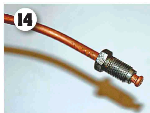
14 The finished pipe flare. Flaring kits cost about £20 upwards and are a useful addition to the tool kit as the copper pipe and fittings can be inexpensively bought in a large range of sizes and thread pitches.
