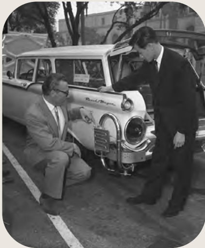
↑ By the early 1970s, air pollution visibly shrouded the streets of Southern California on a daily basis. ➡ The first installation of a catalytic converter was tested on a 1959 Ford Ranch Wagon.
