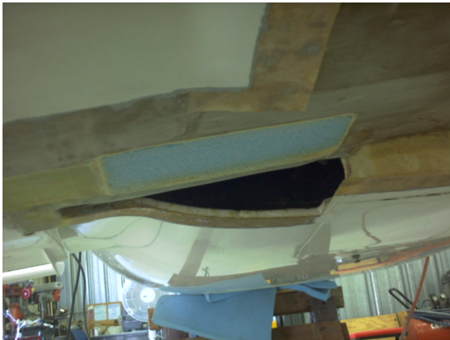
Foam installation bottom of canard
