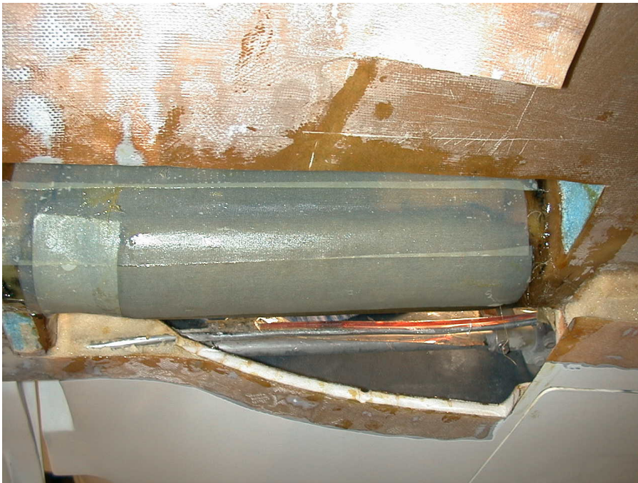
Glass layup bottom of spar
