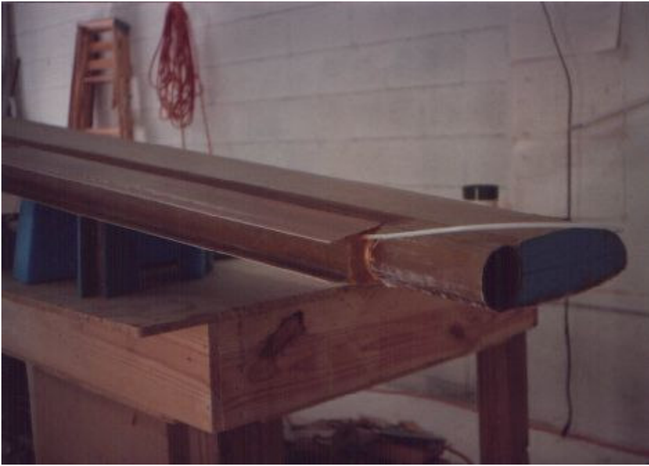
A good view of the canard carbon fiber spar and the slot core being attached. The tube out the end is the brake line.
