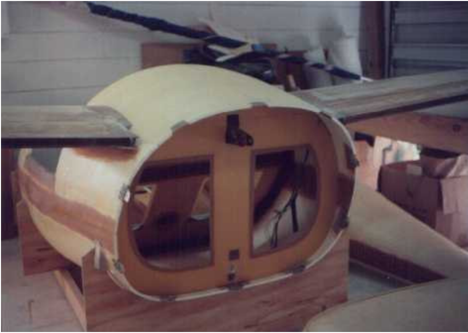
The rear bulkhead and fuselage top are fit in place.
