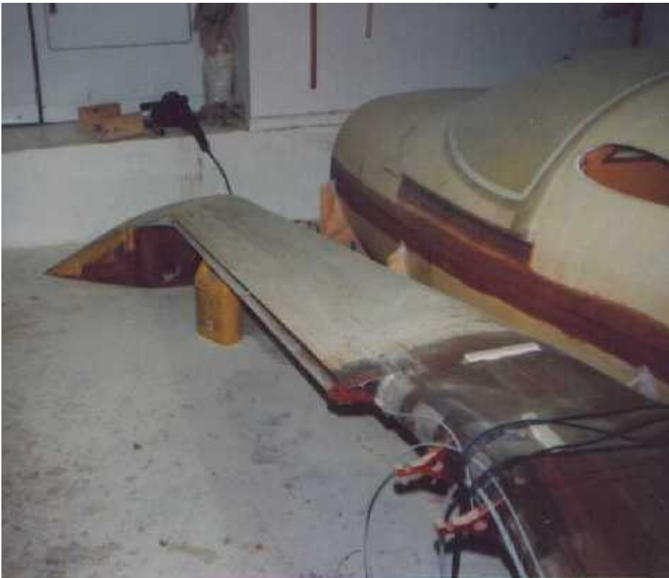
Canard basically ready for installation. Note the fill/prep for paint work has been done up to a few inches prior to the fuselage joint. Ever try to sand the bottom of a
