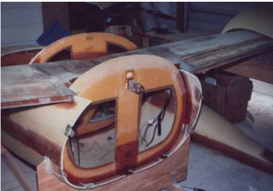
The rear bulkhead is glassed in place
