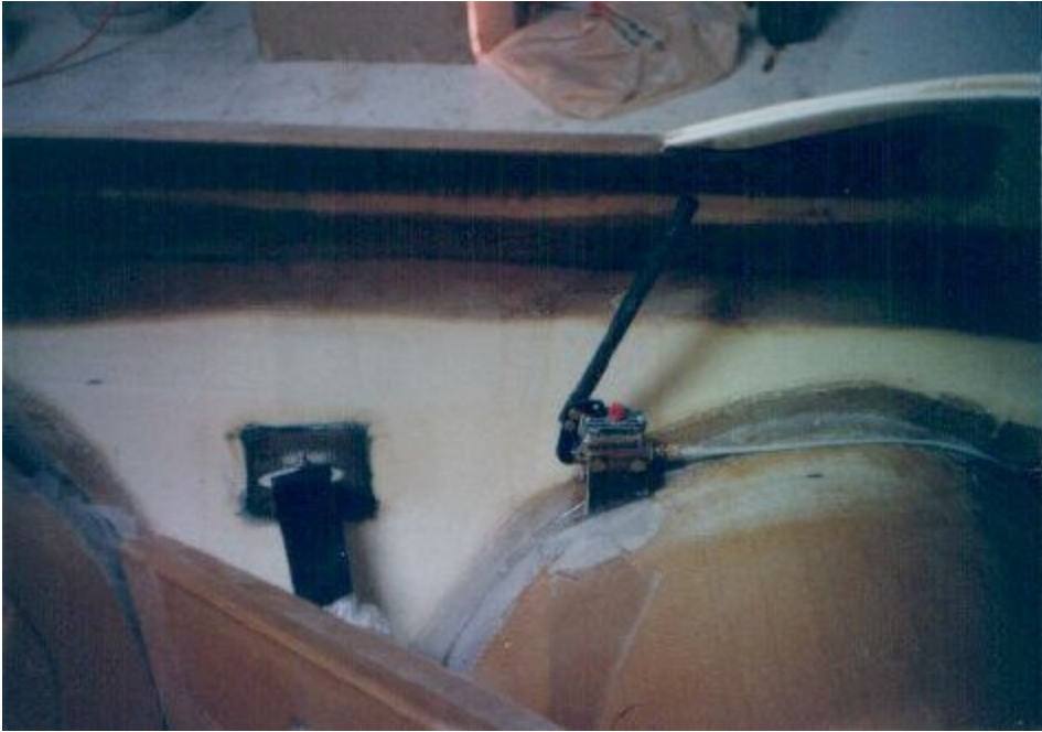
The seat belt and brake master cylinder are installed.
