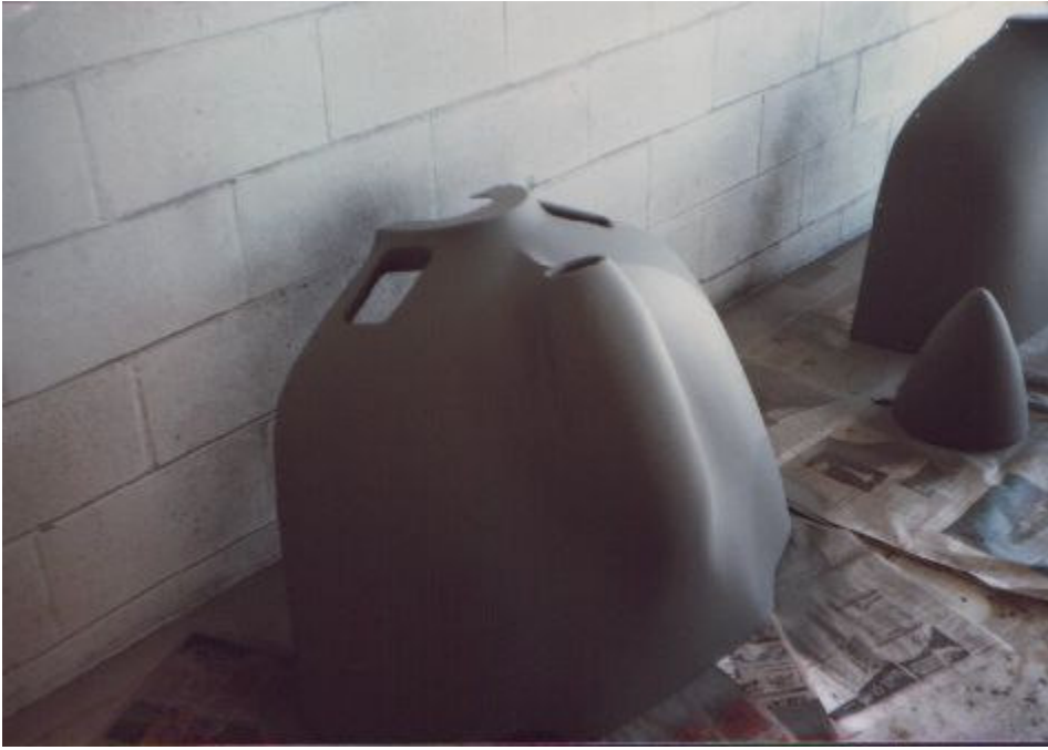
The cowling prepped and ready to paint.
