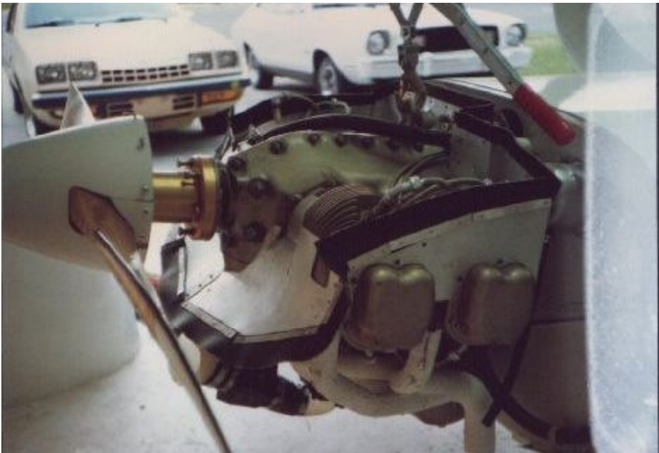
Rubber added to engine baffles. The white coating on the exhaust pipes fell off with a few hours of flight.
