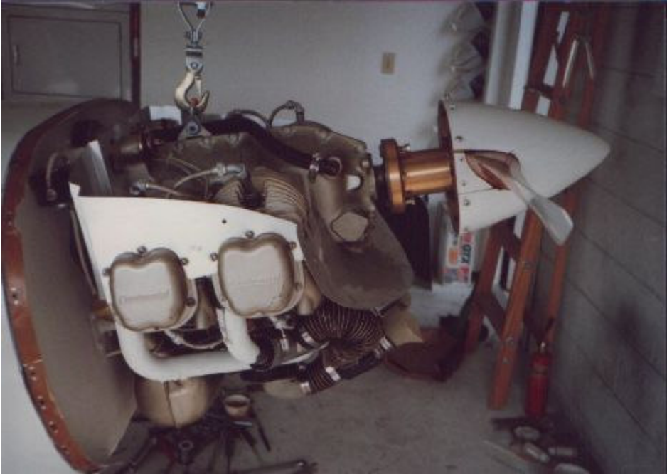
Engine cooling baffles going on.
