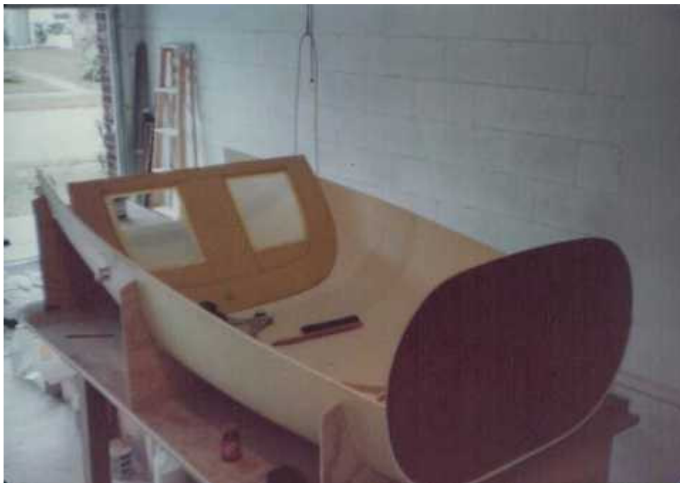
Fuselage Jigging, seatback in place, cutouts for luggage door.
