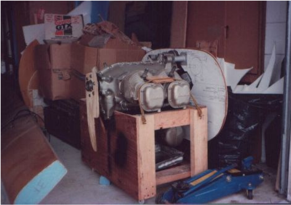
The firewall was fitted to the engine before the firewall was installed.
