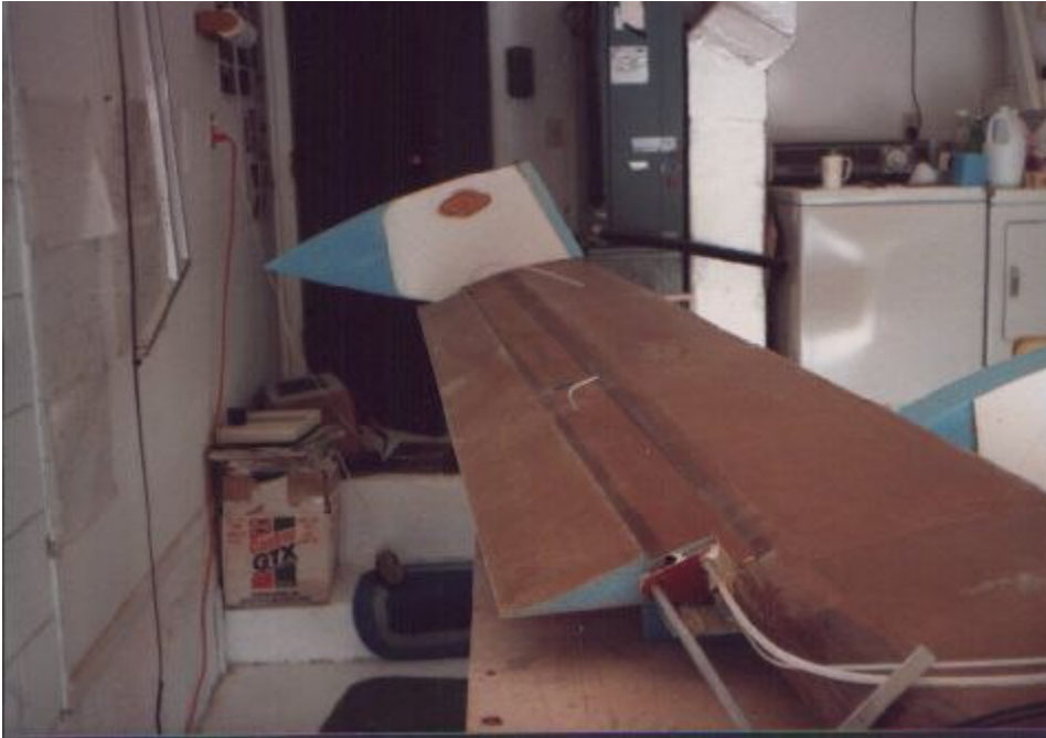
Fitting the wheel pants to the canard. Notice the pitot tube and the fully rigged elevator hinges.
