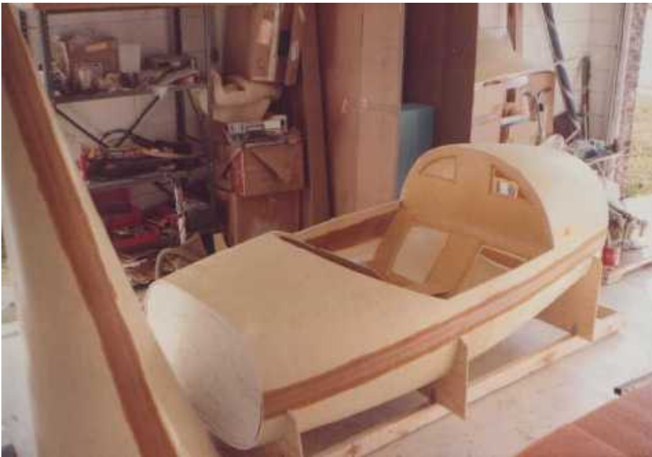
You can see the fuselage shells are joined at the cut line. Instrument panel temporarily in place.
