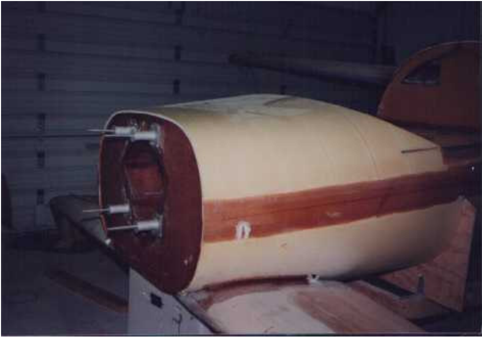
Another view of the firewall installation.
