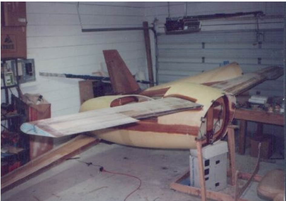
The top fuselage shell is glassed in place.
