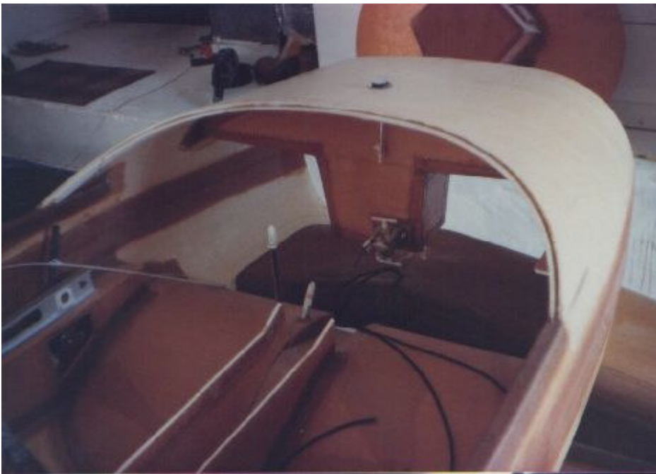
A shot showing that the header tank was installed prior to the firewall.
