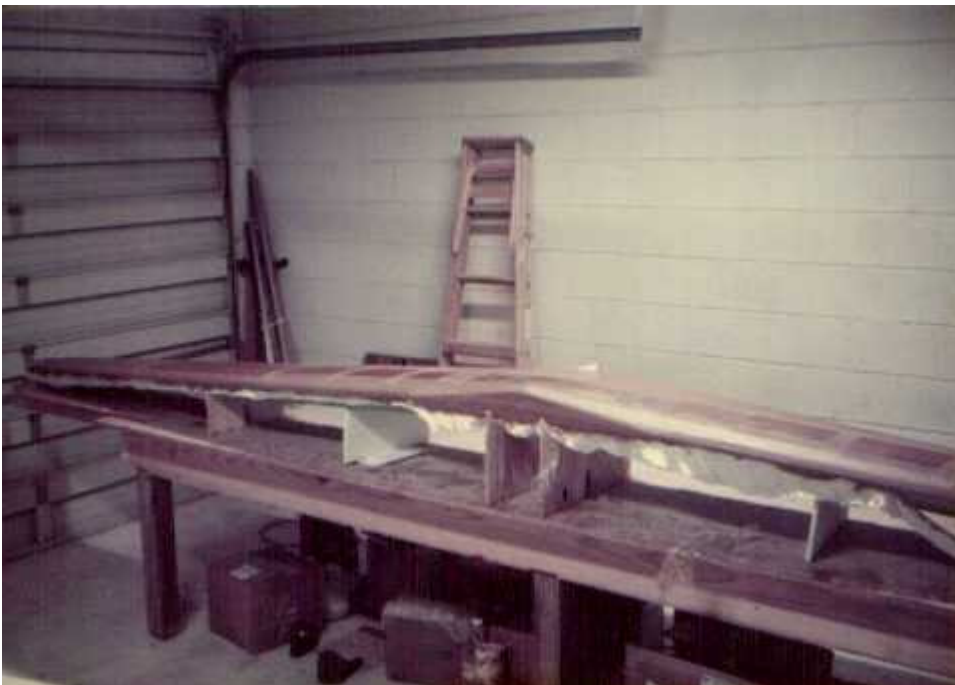
One layup side completed, waiting to cure the epoxy.
