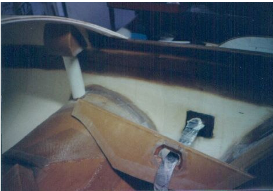
The passenger side seat belt and fuel filler are installed.
