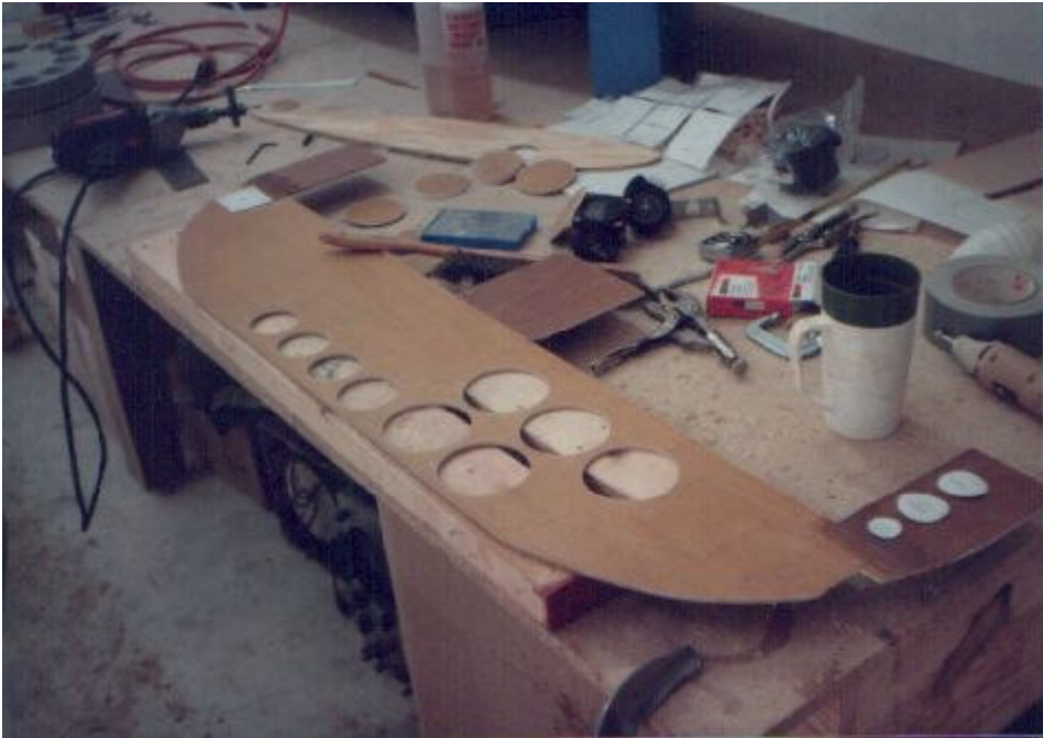
Cutting the instrument panel holes.
