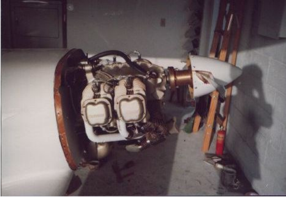
Continental O-200A, rebuilt, 0-time Warnkee Prop
