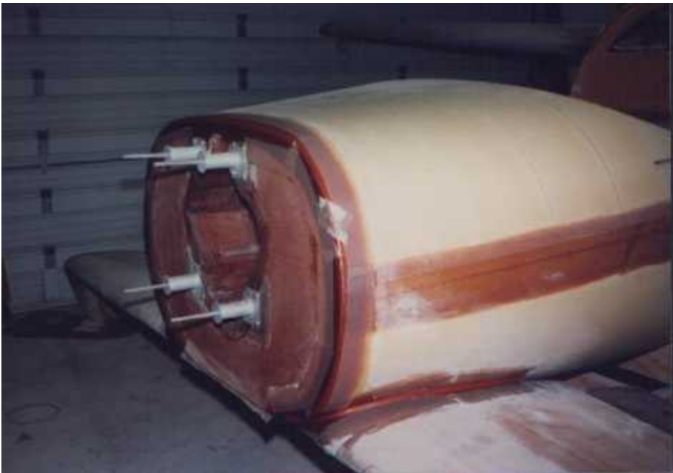
The corner is rounded and layers of fiberglass cloth are used to strengthen the firewall attach. We don't want our engine falling off!
