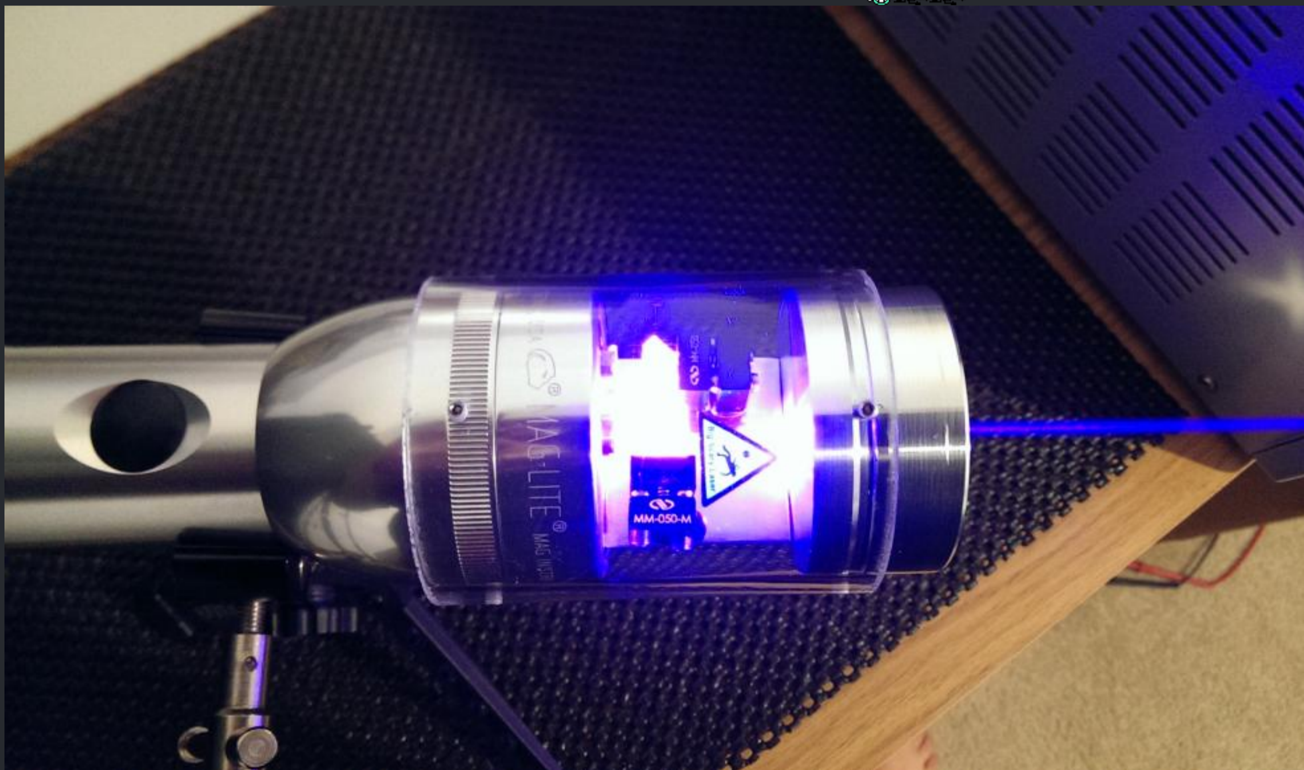
Pretty straight forward I used 2 Groove 2 drivers as I mounted them on some copper pads. I chose the Groove driver, well just because I had so many already going on that I did not want to chance any malice to those honey suckle diodes. 🤪 🎄
