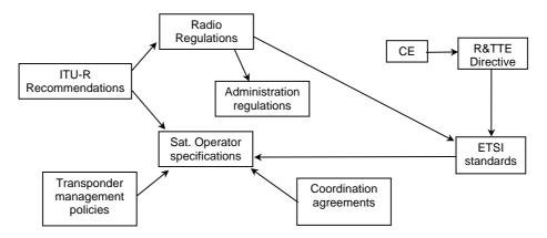
**Figure 1 Families of Interference Protection Standards**
